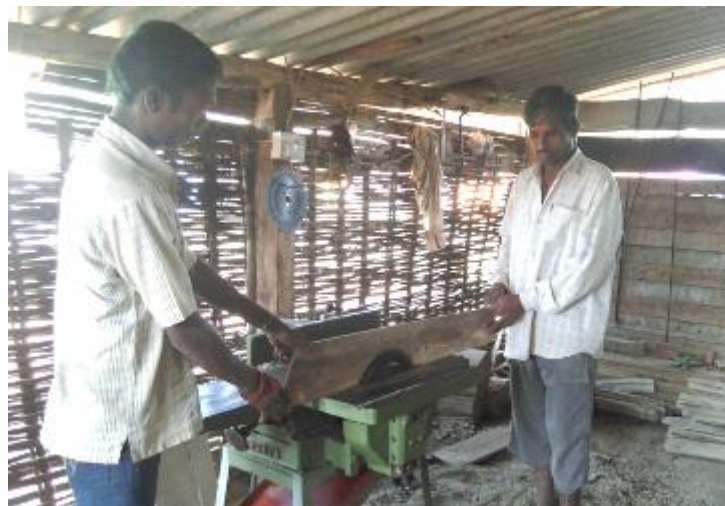
Cutting wood into specific dimensions using a cutting machine
